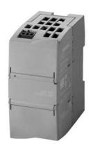
Compact Switch Module CSM 1277 for connecting SIMATIC S7-1200 and up to 3 further nodes to Industrial Ethernet with 10/100 Mbit/s; unmanaged switch, 4 RJ45 ports, ext. 24 V DC power supply LED diagnostics, S7-1200 module incl. electronic Equipment Manual on CD-ROM.
